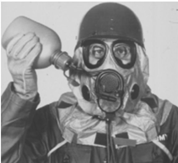
Fig. 16-6. The M17A2 Chemical-Biological Field Mask with drinking tube assembly allows the soldier to drink without unmasking. Soldiers wearing mission-oriented protective posture (MOPP) gear must drink water to prevent heat stress. The drinking tube, essentially a flexible straw, couples with the canteen cap. The soldier holds the canteen upright and inverted, then sips water through the tube. After a few sips, the soldier needs to puff his own exhaled air back into the canteen to equalize the atmospheric pressure without introducing contaminated air. Then he can take a few more sips of water before he needs to equalize the pressure again. Photograph: Courtesy of Chemical and Biological Defense Command Historical Research and Response Team, Aberdeen Proving Ground, Md.
